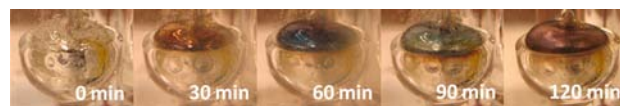
Figure 4. Optical images of a Ga(l) pool electrode immersed in an aqueous solution containing 0.1 M NaOH, 0.1 M \text{Na}_2\text{SO}_4 , and 0.001 M \text{As}_2\text{O}_3 at 90 °C while biased at -1.58 V for 0, 30, 60, 90, and 120 min.
